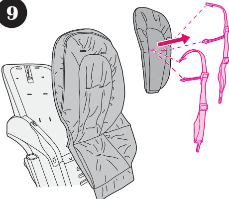
Remove 4 straps from body support as shown.
